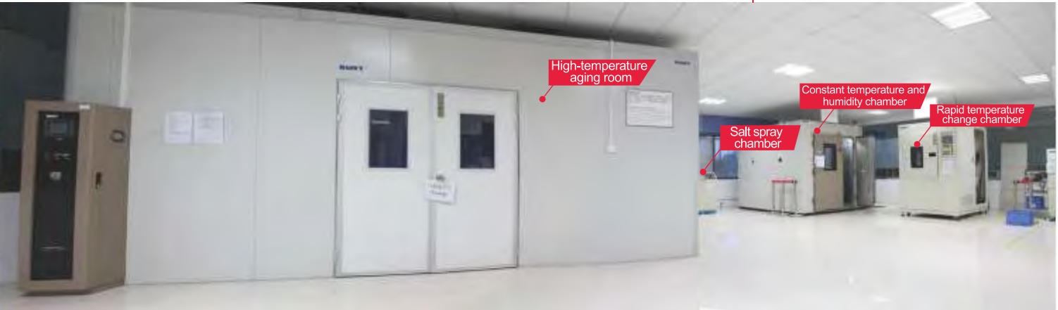
Climate Environmental Laboratory Simulate various extreme climate environments to ensure the quality of products.
