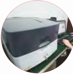
Energy dispersive X-ray fluorescence spectrometer To detect the harmful materials, according to the demand of EU standard
