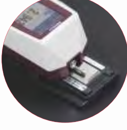
Roughness detector imported from Japan , to test the roughness of metal surface
